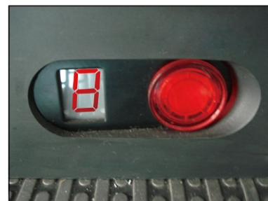
Fault Display for S and F Type
